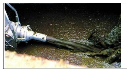
Lower the pump until the stirring nozzle dives into the floating layer.
