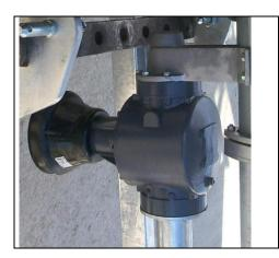
The gear box is filled with 2 liter gear oil type Spirax 90 EP up to the Kontrollschraube. Change the oild for the first time after 50 operating hours, every further change has to be conducted after 800 to 1000 operating hours.
