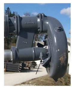
Inspect the cutting edges of the knives. Theiy are constructed in a way that they can be used four times before they have to be sharpened again.
