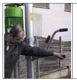
The stirring device has three levers.
